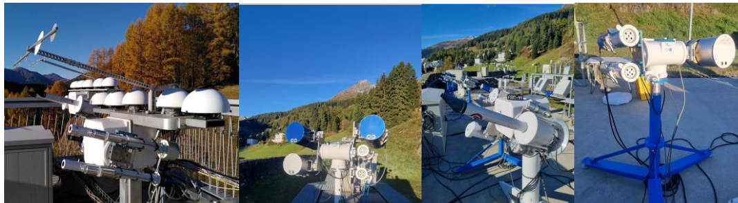
Figure 1. Spectroradiometers involved in the FRC-VI campaign in Davos. From left to right: (1) PMOD/WRC BTS-VL and QASUME (reference), (2) PMOD/WRC PSR Triad with two PFRs, (3) CIEMAT BTS-VL on the DWD tracker, and (4) DWD instrument suite at FRC-VI with two PFRs and PSR#004 on a PMOD/WRC tracker.
