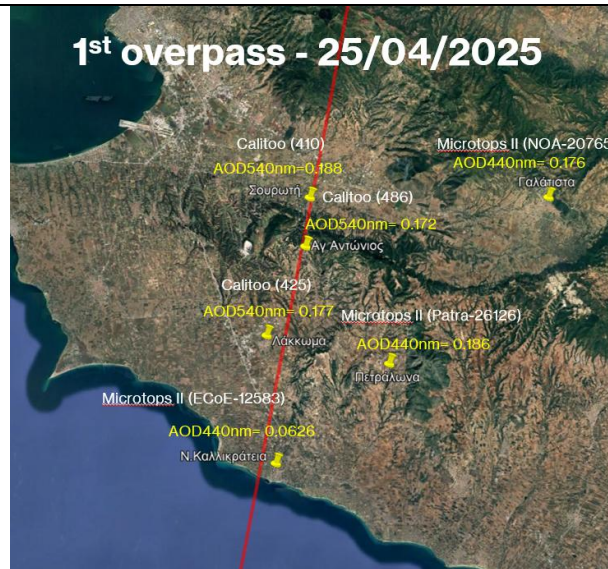
Figure 1. EarthCARE overpass path and locations of handheld sun-photometer measurements (indicated with pins), along with the mean calibrated AOD values per instrument at 440 nm for Microtops II and 540 nm for Calitoo instruments.
