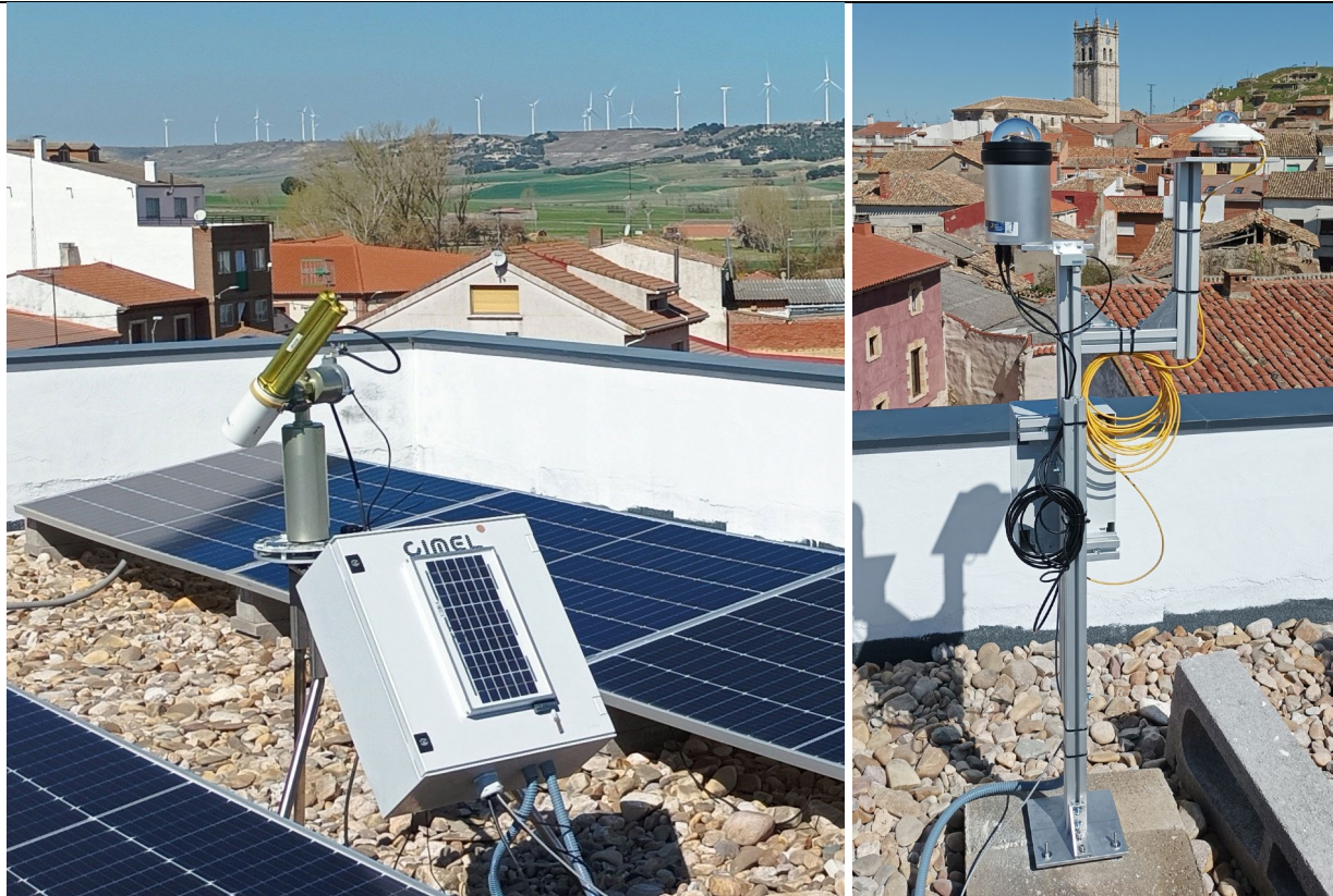
Figure: An AERONET CE318-T sun/sky/moon photometer (left), and an OMEA-3C-TF all-sky camera collocated with an SMP10-V global pyranometer (right), all of them in the rooftop of the “Centro Cultural Polivalente” centre of Baltanás (Palencia, Spain).
